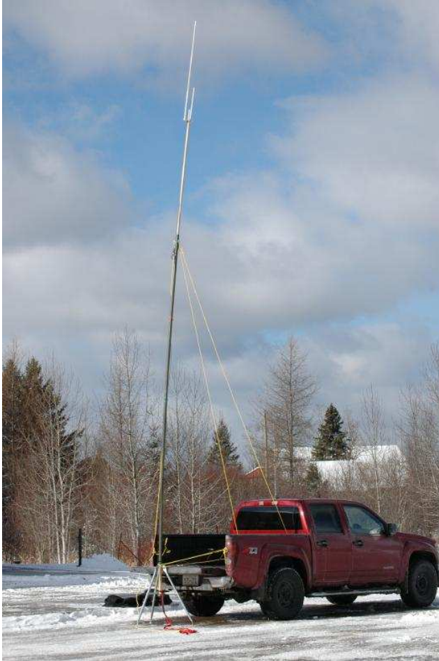
This was the mast and antenna at Killaloe. It consisted of 4 sections of fiberglass mast, a length of wood dowel and an Arrow dual band J-pole. (It was guyed to lean against the wind.)
