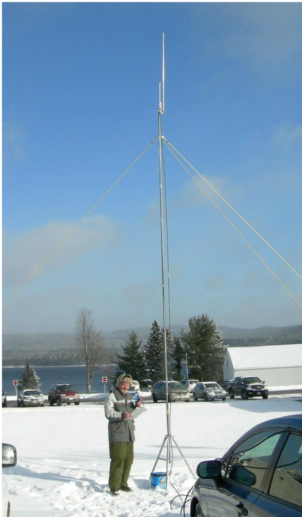
This antenna was at the Deep River town hall. The mast is four 5 ft sections of swaged fence top rail and the antenna is another Arrow dual band J-pole.
